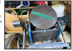
rollers. The rollers transfer ink from the disc onto the die, which then gets pressed into a platen that holds the paper.
